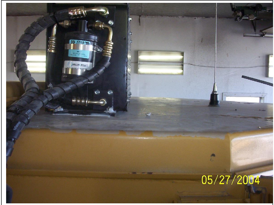
Condenser mounted on a D5H. Similar set up for the 816B
