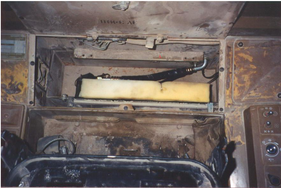
Evaporator in place for 816B with hoses.
